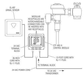
One 50 VA Transformer serves up to ten (10) OPTIMA Closet/Urinal Flushometers. Specify number of transformers required accordingly.
