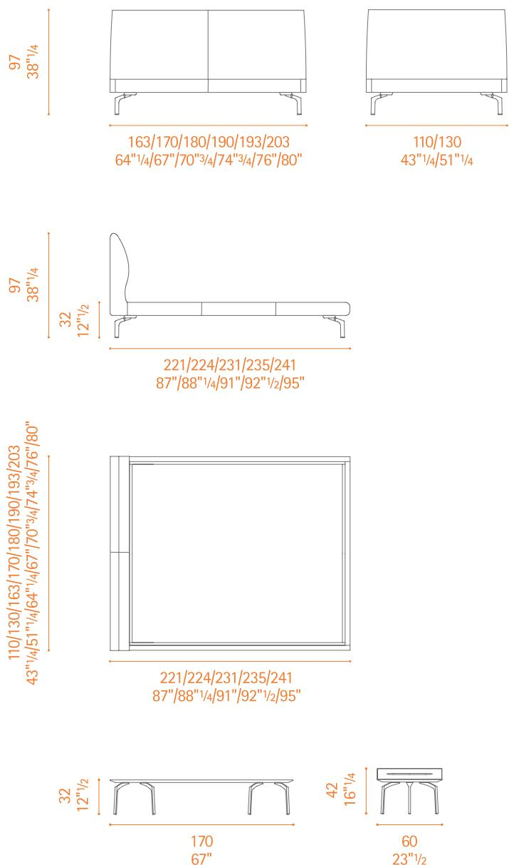
1:50 scale. All dimensions and sizes are in centimeter and inches; dimensional variations of +/- 2% are possible.
