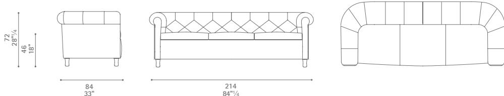
1:50 scale. All dimensions and sizes are in centimeter and inches; dimensional variations of +/- 2% are possible.
