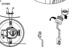
5. UNPLUG CONNECTOR AND SCREW THREADED BASE INTO CAN SOCKET
