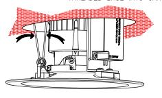
8. LIFT LED RETROFIT TRIM AND POSITION SECOND TORSION SPRING IN CAN
