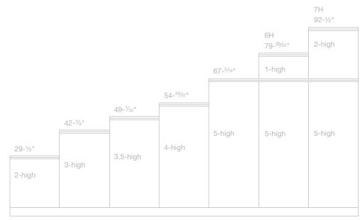
Xsite frames are available in five different base heights and can be built up to 80" and 93" tall by adding one or two stackers. Frames can be extended in three-inch increments. So, offices can be sized as needed
