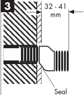
6. Fasten the thermostatic mixer onto the S-unions using the union nuts. Align the unit and tighten the nuts (be careful not to damage the chrome finish). The S-unions allow inaccuracies to be compensated for.
