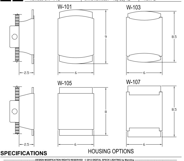
HOUSING: CONSISTS OF 0.090 THICK FABRICATED, LASER CUT ALUMINUM, WITH AN ELECTRO-GALVANIZED STEEL MOUNTING PLATE.
