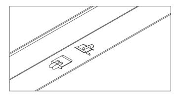
Continue to install sections of molding along this first wall by butting factory-cut ends together. Trim shorter sections of molding carefully to maintain 12" from the cut end to the center mark of the first lock.
