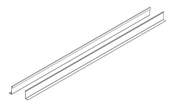
Ultima Plank panels with Shiplap edge are directional. Once the first panel is installed in the grid, all others must be installed in the same direction. Tegular cuts must be provided on all panel edges that meet the Locking Angle Molding.
