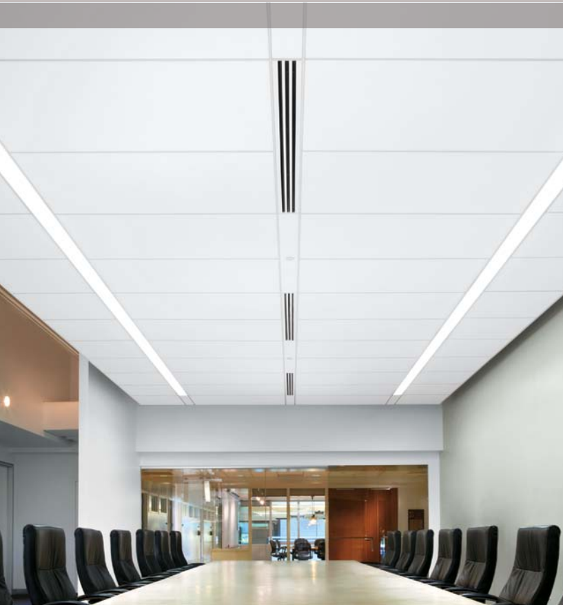
TechZone Ceiling System with 30" x 60" Optima Tegular Field Panels and 6" Wide Technical Zones for Continuous Lighting
