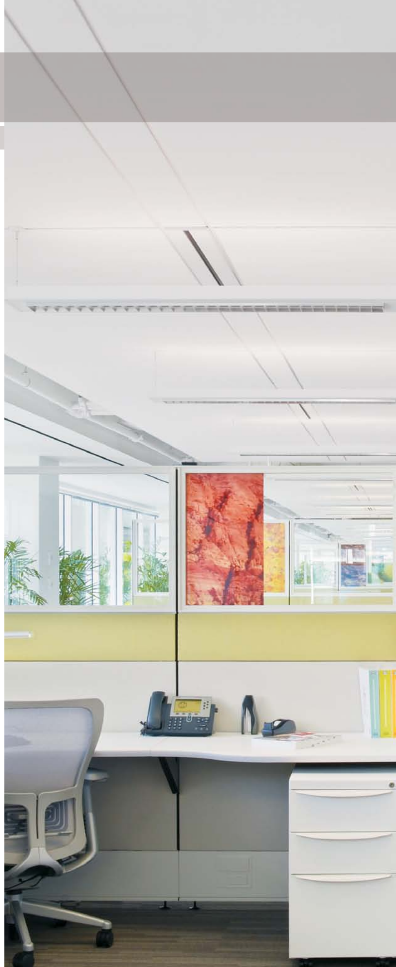
TechZone Ceiling System with Optima Tegular 4' x 4' Field Panels and 6" Wide Technical Zones
