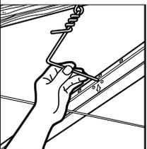
Pull each hanger wire through a round hole below the bulb of the main tee and bend up, twisting the end 3 turns (within a 3" span).
