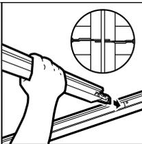
**Install cross tees.** Insert tabs into slots in the main tee. Where two cross tees occupy the same slot, insert the second cross tee to the left of the first cross tee.
