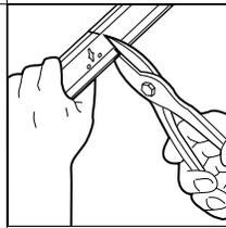
Cutting tees is easiest with metal snips. First, cut the bulb and stem, then bend the tee at the cut and snip the face flanges. Sand or file rough edges. If metal snips are not available, use a hacksaw to saw down from the bulb through the stem and flanges; file rough edges smooth.
