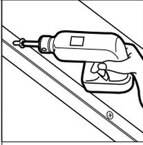
**Install wall angles.** Align the top of each wall angle along the chalk line. Space screws every 2' o.c. or closer.
