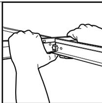
**To remove a cross tee,** push up on the main tee and twist away until the cross tee pops out.
