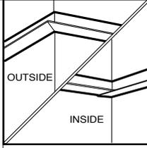
**Cut the corners.** At outside corners, miter wall angles to 45 degrees. At inside corners, cut angles to 90 degrees and butt together.
