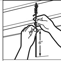
**Install hanger wires.** Install lag screws at 4' intervals along the main-tee string lines. Attach a hanger wire to each screw and cut 6" below the string line. Bend each hanger wire to a 90-degree angle 3/4" above the string line.
