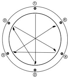
Use several rotations of the following sequence to tighten firmly the lens ring screws, to 20 in/lbs. max.
