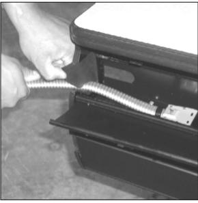
Extend the jumper through end cap as shown by feeding conduit through the slit in the rubber.
