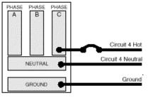
In the four-circuit 3+1 schematic, circuits 1, 2, and 3 are distributed from the first circuit panel and are supported with one shared neutral and one shared ground. Circuit 4 is distributed from a second circuit panel and is supported with a separate neutral and ground.
