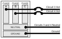
In the four-circuit 2+2 schematic, circuits 1 and 2 are distributed from two different phases from the first circuit panel and are supported with one shared neutral and one shared ground. Circuits 3 and 4 are distributed from a second circuit panel and supported by their own shared neutral and ground.
