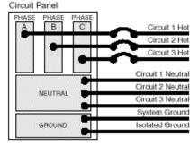
On a single 3-phase circuit panel, three circuits are distributed as shown.
