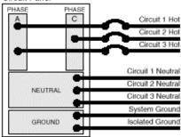
On a split-phase circuit panel, three circuits are distributed as shown.
