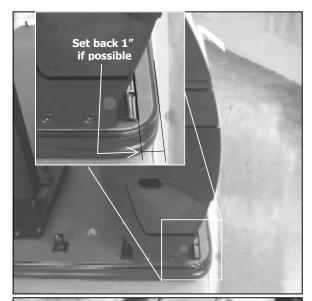
1. With the table upside down on a soft, protected surface, attach Juice with the screws provided.
