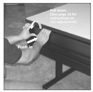
2. Carefully turn the table right side up and pull the jumper through the end cap.
