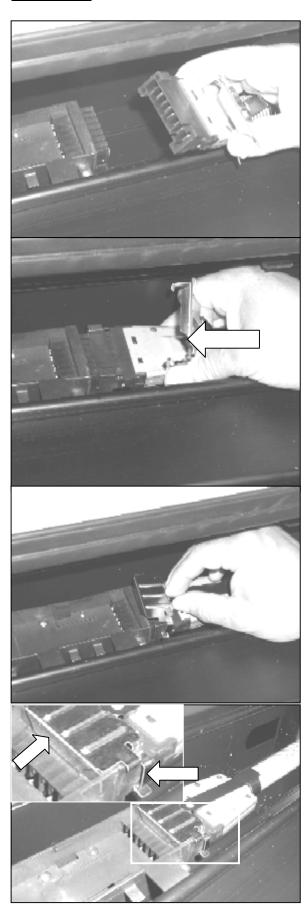
3. Connect the jumper from one table to the power block on the next table.
