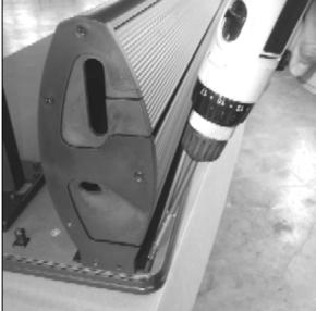
The screws should be inserted at an angle so that the drill does not scrape the unit while driving the screw. Drive the screw head flush with the flange surface.
