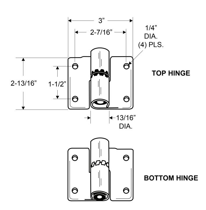
**NOTE: HINGE THICKNESS AT 3/32"** 7151, 7152 TOP HINGE ONLY, 7161, 7162 BOTTOM HINGE ONLY TOP AND BOTTOM HINGE DIMENSIONS ARE SAME
