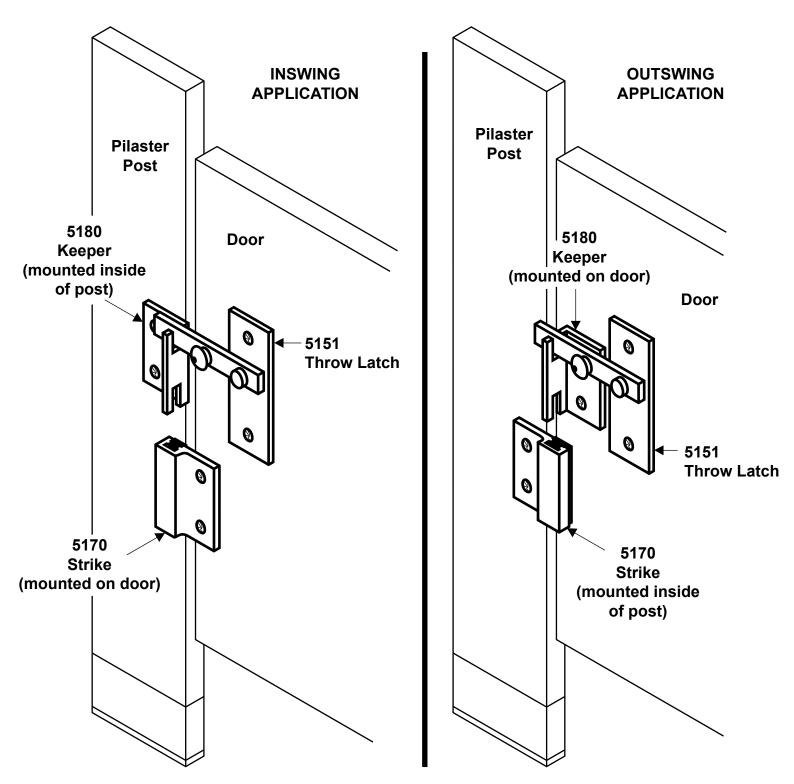
NOTE: 5400 DOOR PULL MOUNTED ON OUTSIDE OF DOOR (HOLES ARE TO LINE UP WITH HOLES ON MOUNTING PLATE OF THROW LATCH)
