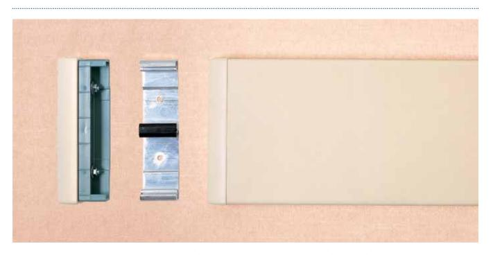
The **KOROGARD** C860 Crash Rail is 8" (203.2mm) high installed with 2" (50.8mm) wall brackets 16" O.C. The C860 Crash Rail provides an impact-resistant barrier to damaging carts and gurneys. **KOROGARD** rugged durability makes the C860 Crash Rail best suited for medium- to high-impact areas.
