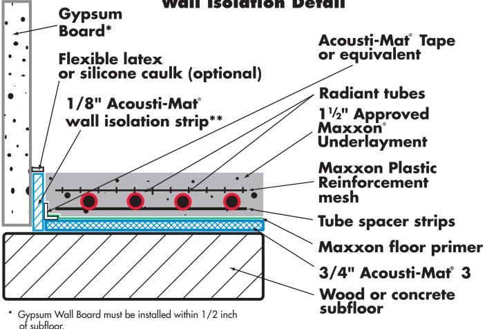
\*\* Acousti-Mat® Wall Isolation is installed around the perimeter of the entire room to receive Acousti-Mat 3, and around any floor penetrations such as toilet collars, electrical, plumbing, etc.
