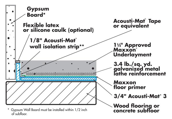
\*\* Acousti-Mat® Wall Isolation is installed around the perimeter of the entire room to receive Acousti-Mat 3, and around any floor penetrations such as toilet collars, electrical, plumbing, etc.
