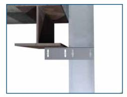
Align studs to SLS for plumb wall assembly.
