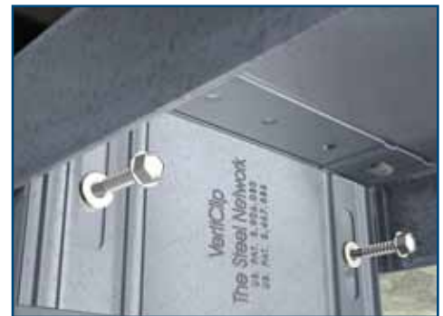
Attach VertiClip through Step Bushings to wall studs with self-drilling screws provided.
