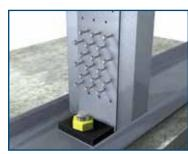
Secure clip to stud with required amount of symmetrically placed #12 screw fasteners.
