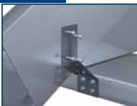
To install the StiffClip RT, place one end flush against the roof framing member with the other end abutting the wall framing member.
