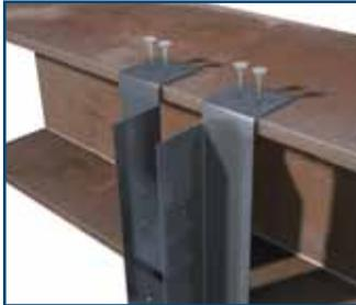
Attach StiffClip JH to beam with required fasteners. Use blocking behind clip if clip length is less than beam depth.
