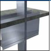
Place StiffClip FS flat against aligned wall studs.
