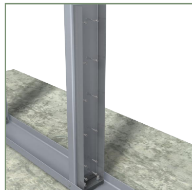
Attach MidWall™ 24" to the stud web with #12 screw fasteners through guide holes (fill all holes in the vertical MidWall™ leg).
