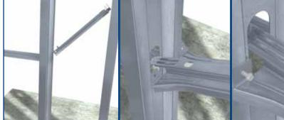
Twist BuckleBridge into stud punchout and insert tab into slot of previously installed BuckleBridge.
