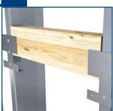
Rest wood piece on shelf legs and attach to clip with required number of screws through guide holes. For higher loads, attach Backlt® to the stud web through a guide hole in the interior leg.
