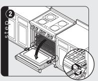
Open door completely. Reinstall hinge trim.
