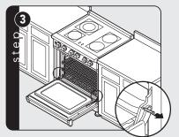
Remove pins from hole in hinges.
