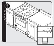
If the door needs to be adjusted, loosen hinge trim screws (see step 2). Adjust the screws located between the door and kickplate using a 5/32" hex head allen wrench. After adjustment, tighten hinge trim screws.
