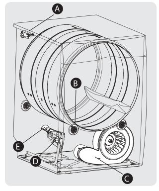
E. GAS BURNER (Gas models only.) When the burner is operating, there may be sounds generated as the air flow mixes with the gas flame. This noise is normal and will only occur when the gas is ignited in the combustion tube.
