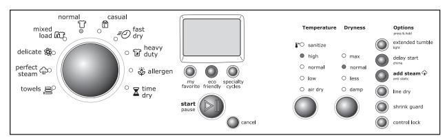
Turn the cycle selector in either direction to the cycle desired. The indicator for that cycle will be illuminated. Press on the cycle selector knob to extend it or return it flush to the console.
