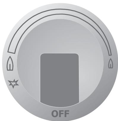
In the event of an electrical power outage, the surface burners can be lit manually. To light a surface burner, hold a lit match to the burner head, then slowly turn the Surface Control knob to
