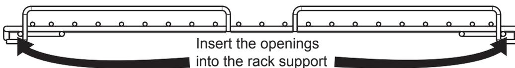
**⚠ WARNING** Always arrange the oven racks when the oven is cool (prior to operating the oven). Always use oven mitts when using the oven.
