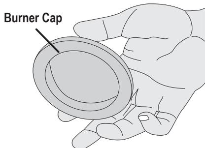
Place a burner cap on each burner head, matching the cap size to the head size. The cap for each burner has an inner locating ring which centers the cap correctly on the burner head. Be sure that all the burner caps and burner heads are correctly placed **BEFORE** using your appliance.
