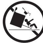
To reduce the risk of tipping of the range, the range must be secured by properly installed anti-tip bracket(s) provided with the range. To check if the bracket (s) is installed properly, remove the lower panel or storage drawer and verify that the anti-tip bracket (s) is engaged. Refer to the installation instructions for proper anti-tip bracket(s).
