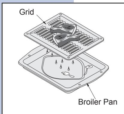
To make cleaning easier, line the bottom of the broiler pan with aluminum foil. **DO NOT** cover the broiler grid with foil.
