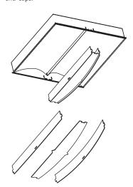
Acrylic diffuser shield is easily removed for lamp access and maintenance.
