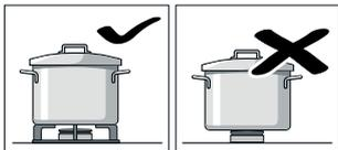
Place the pots or pans on the pan support, never directly on the burner.
