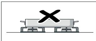
Do not heat a cooking vessel (e.g. roaster, pan, grill stone) on more than one burner at the same time. The resulting heat accumulation will damage the appliance.
