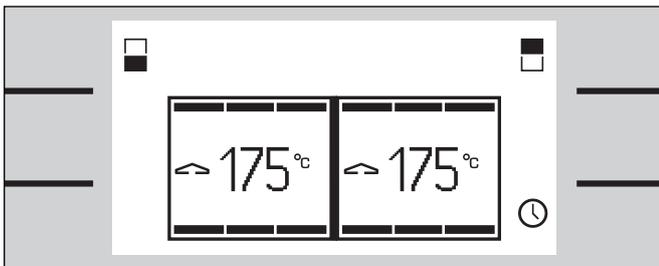
When turning a knob of one of the ovens, the settings of this oven are shown on the display. After a short while the display for both ovens appears again. You can also touch the
