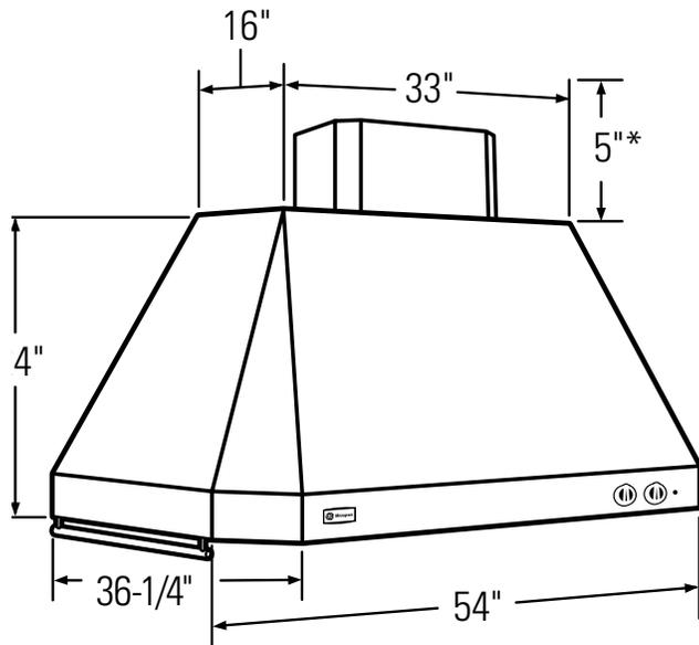
\*5" for ceiling heights of 7' 11" to 8' 5" using the supplied support frame and duct cover.
