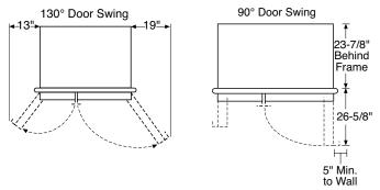
Allow minimum clearances for freezer door and fresh food door for a full 130° door swing and to allow for pan removal.
