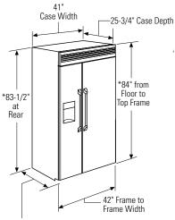
\* Shipping height. The refrigerator can be adjusted to fit into a cutout that is 83-1/2" min. to 84-1/2" max. height. Note that the top case trim at the front is 1/2" higher and will overlap upper cabinetry or soffit. Use leveling legs and wheels for a maximum 1" height adjustment.
