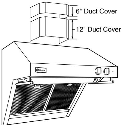
Decorative duct covers are available in 6" and 12" heights. Duct covers may be stacked, in various combinations, to conceal the ductwork running from the top of the hood to the ceiling.
