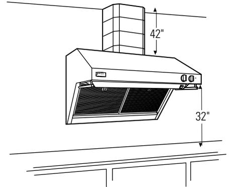
**10 ft. ceilings:** When the hood is installed 36" above the cooking surface, order three 12" and one 6" duct cover accessories.
