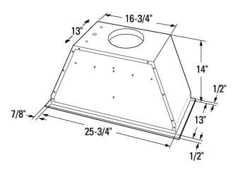
The bottom edge of the insert sleeve has a 7/8" wide flange on the sides and a 1/2" wide flange on the front and back.
