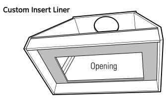
The custom canopy must be sized to fit the insert sleeve. Construct the canopy with an opening that is:  $26"W \times 13-3/16"D$
