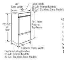
\*Shipping Height. The refrigerator can be adjusted to fit into a cutout that is 83-1/2" min. to 84-1/2" max. height. The top case trim at the front is 1/2" higher and will overlap upper cabinetry or soffit. Use leveling legs and wheels for a maximum 1" height adjustment.
