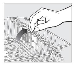
Raise the rack to make room for tall glasses. Lower it to double stack smaller pieces.
