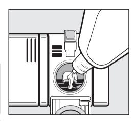
Pour liquid rinse aid into the reservoir until it is visible on the surface of the screen.
