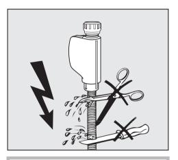
Do not cut the intake hose. It contains electrical wiring. If the hose is cut, the dishwasher will not work. There will be a water leak and you could be injured. If the hose is too long, coil it neatly and place it behind the machine.
