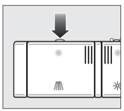
Press the latch on the detergent dispenser. The flap will spring open.
