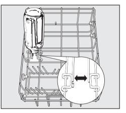
Place the bottle holder in the lower basket as shown in the illustration. If placed anywhere else, water from the spray jets will not reach all surfaces. The bottles will not be properly cleaned.
