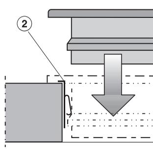
For granite countertops, the spring clips, ②, must be placed in position and secured with double-sided tape. In addition, coat the edges of the spring clips with silicone sealant. The screws are not needed for granite countertops.
