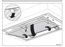
■ To remove the grease filters pull the locking clips forward. Lower the filter 45° unhook it at the rear and take it out. Support the grease filters so that they do not fall onto the cooktop.
