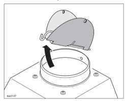
The hood comes equipped with a **non-return flap.** This flap automatically closes when the hood is turned off so that no exchange of outside air and room air can occur.
