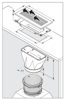
If site conditions are not suitable for the hood to be used for air extraction, the appliance must be converted for recirculation using the following installation kit. It can be ordered from your Miele dealer or the Technical Service Dept.
