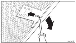
If the filters are incorrectly installed, insert a small screwdriver into the slit along its edge to disengage it from the casing.
