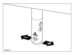
Use the joystick to select the desired time. Press it to the left for a shorter operating time, to the right for a longer operating time.
