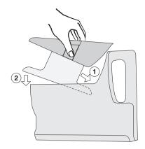
Reinsert the insert into the steam generator only when both parts are dry. Place the insert in at an angle (1) then lower the side with the opening (2).
