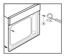
Push the appliance into the niche. After aligning the oven it must be secured in position. Open the oven door and using the two supplied screws (9), secure it to the cabinet through the holes on either side of the vertical oven trim. Installation, repairs and other work by unqualified persons could be dangerous.
