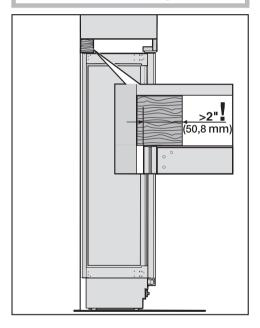
Cut a wooden beam (cross section min. 3" x 4" [75 mm x 100 mm]) to the required length. The length is equal to the width of the installation niche.
