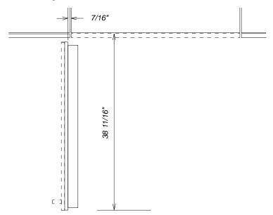
**NOTE**: Additional space needed depending on thickness of front panels and handle used
