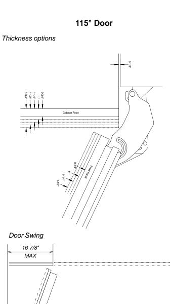
**NOTE**: Additional space needed depending on thickness of front panels and handle used
