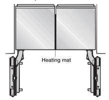
If the appliances are installed directly next to each other (without a partition), they will need to be attached together. A heating mat must also be installed. This will help avoid condensation and prevent damage.
