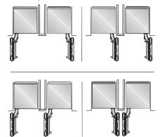
The minimum thickness of the partition is  $\frac{5}{8}$  (16 mm).
