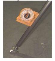
4. If brace spread has been specified in the ordered, place an angle indicator on the upper brace assembly parallel to the platform and rotate the brace until required angle is obtained.
