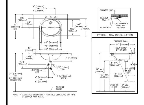
IMPORTANT: These dimensions are nominal and may vary within the range of tolerances established by ASME Standard A 112.19.2
