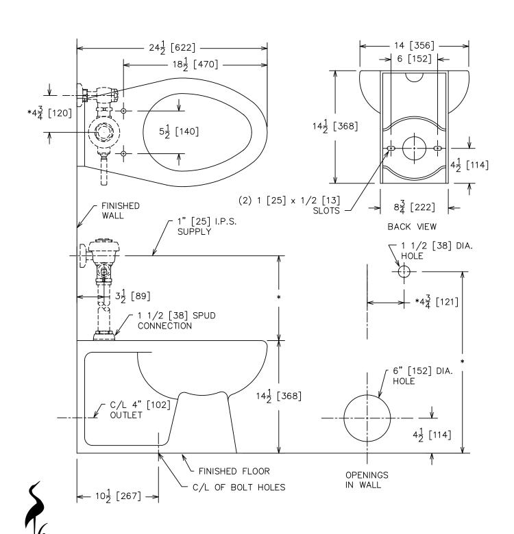
NOTE: \* VARIABLE-CHECK WITH MANUFACTURER OF FLUSHVALVE FOR PROPER ROUGHING-IN DIMENSION.
