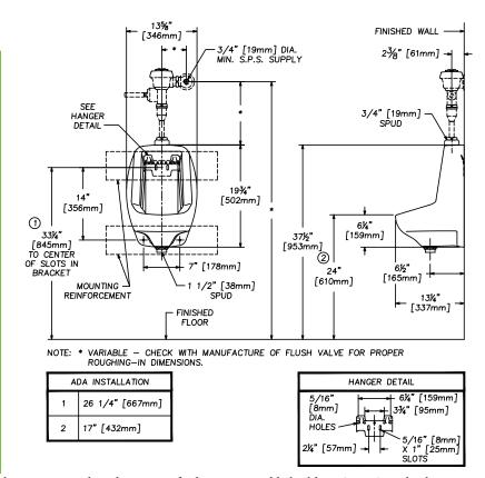
IMPORTANT: These dimensions are nominal and may vary within the range of tolerances established by ASME Standard A 112.19.2
