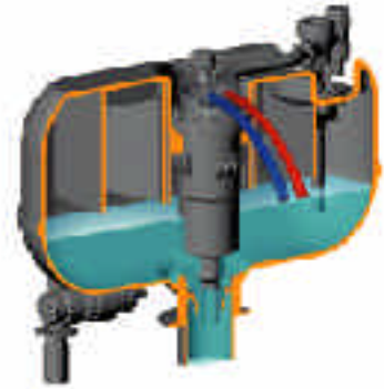
C. Air pressure acts as a powerful piston to drive the water from the vessel into the bowl
