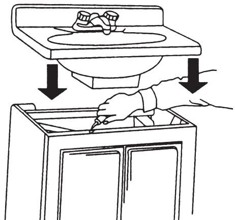
Remove the vanity top from the carton and place on the vanity for a trial fit. Insure the vanity top is the proper size. Check to make sure there is ample room for the fittings, water supply and drain connections.
